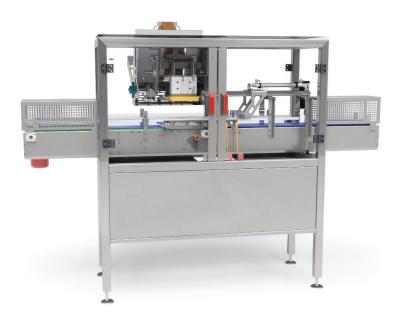
The KA100 KlippaPly unit applies KlippaKan clips automatically to the cans as they travel from the customers accumulation conveyor in rows of 2, at a rate of up to 120 cans per minute, discharging the cans to downstream equipment.
